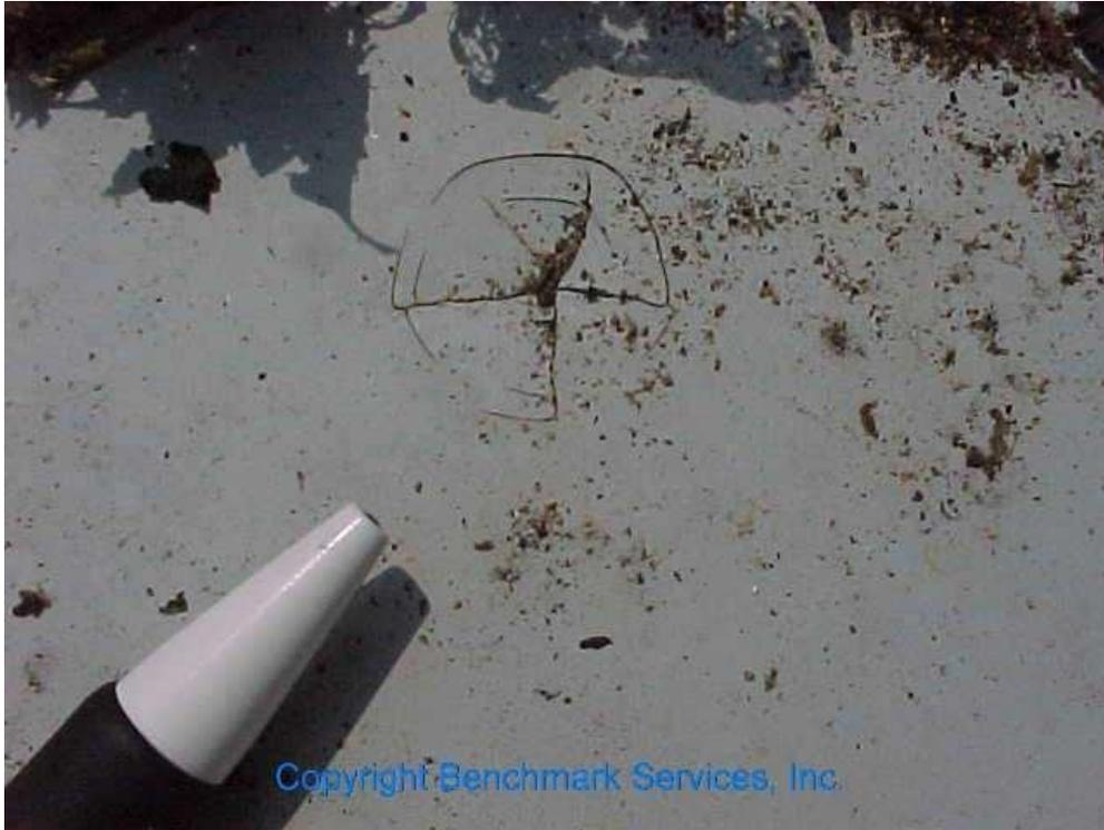
**Figure 7 - Non-Reinforced PVC Membrane Damaged By Small Hail**
